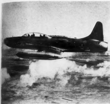
Cover—The F-94 all-weather fighter-interceptor, manufactured by Lockheed Aircraft Corporation, is an active participant in the Korean war theater. It is armed with four 0.50-cal. machine guns located in the nose.
